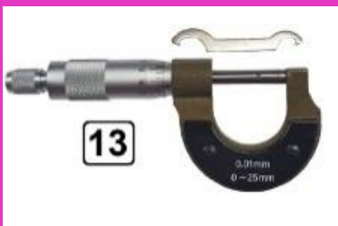
13. WG-025-EMM External Micrometer (Range 0- 25mm , 0.01 mm)
